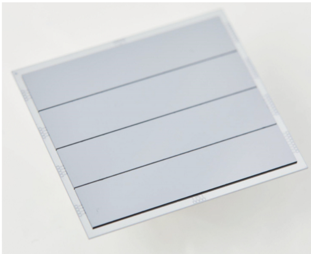
Rigetti's proprietary multi-chip architecture enables larger quantum processors to be constructed by assembling individual chips together, thereby supporting multiple quantum processor generations of increasing scale and performance
